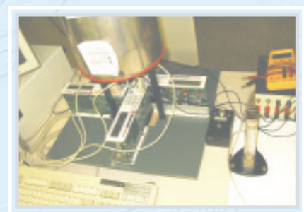
The #7.850 tower connected with four spectrometers. There is still the combination of a tower and two environmental spectrometers.
